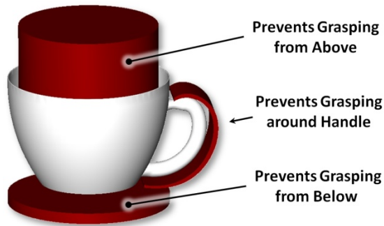
Fig. 5. Coffee cups are not usually grasped from their bottom or inner surfaces, thus the corresponding obstacle prevents access to those areas.
